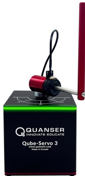
Figure 2. Qube-Servo 3 with the rotary pendulum attachment. The inertia disk is used for the beginner motor and measurement activity described below.
