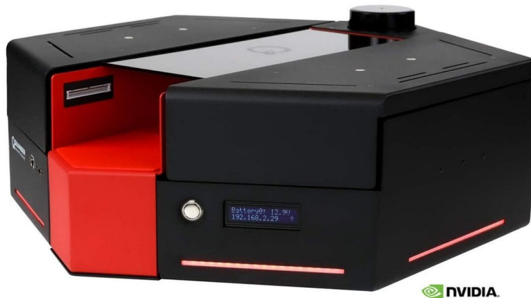
Figure 8. QBot Platform. This mobile ground robot supports investigations of movement, sensing, and navigation concepts.
