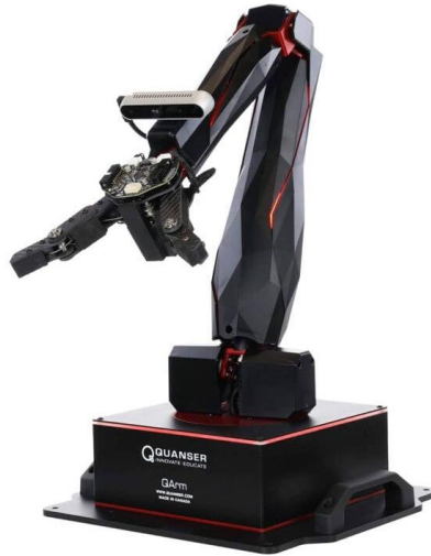
Figure 6. Quanser QArm. The arm, gripper, camera, and base provide a physical reference for the manipulation and sensing activities.
