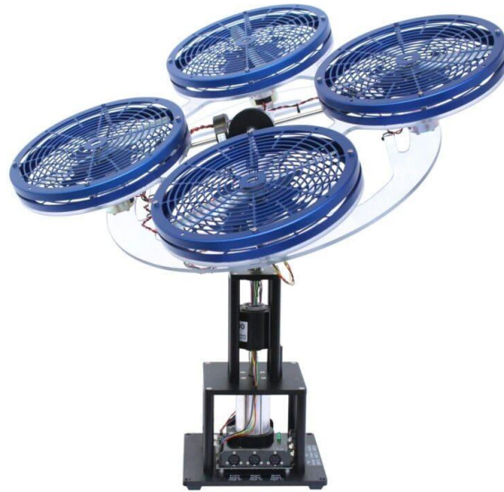
Figure 10. 3 DOF Hover. Source: Quanser product documentation. This resource extends the laboratory discussion beyond the four core 2026 group platforms.
